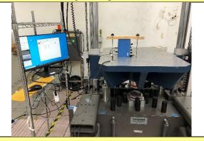
Mechanical Shock Test (+X axis)
